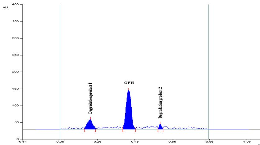
**Fig. 3: Representative densitogram after alkali treatment with degradation products at  $R_F = 0.23$  and  $0.56$**
