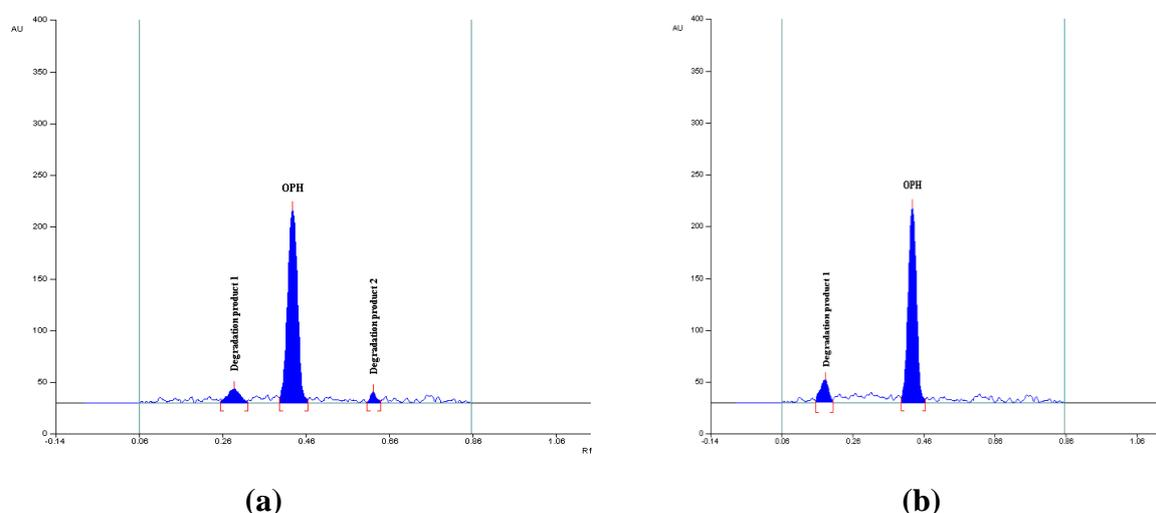
**Fig. 6: Photo degradation densitogram obtained after exposure to (a) UV light ( $R_F = 0.29$  and  $0.63$ ) (b) Fluorescence light ( $R_F = 0.18$ )**
