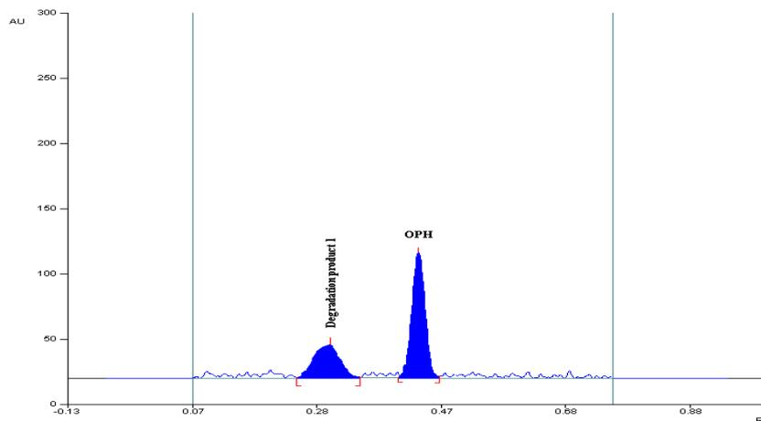
**Fig. 5: Representative densitogram obtained after neutral degradation with degradation product at  $R_F = 0.32$**
