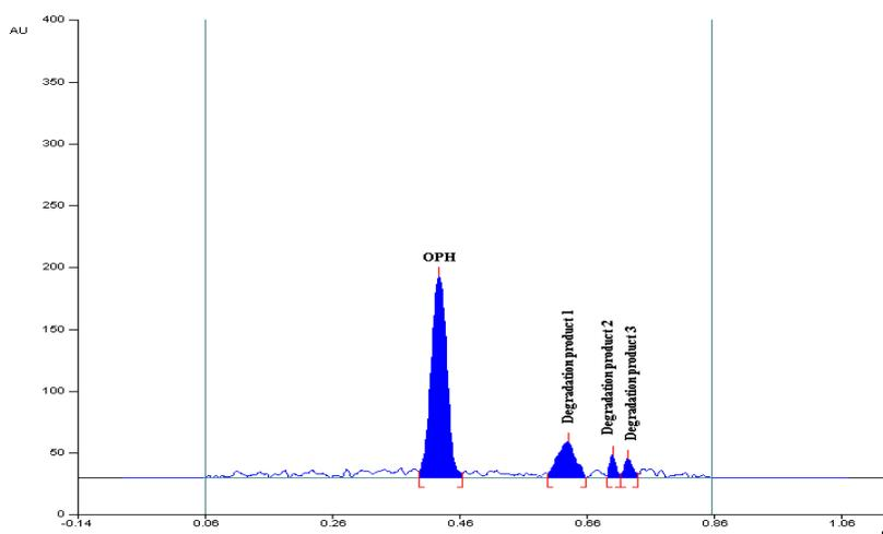
**Fig. 4: Oxidative degradation densitogram with degradation products at  $R_F = 0.62$ ,  $0.70$  and  $0.73$**
