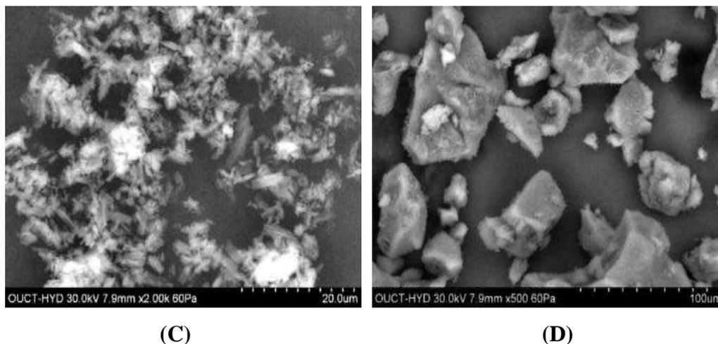
**Fig 9: Scanning Electron Microscopy of (A) Febuxostat, (B) soluplus, (C) Physical mixture (FBXS2), (D) Solid dispersion (FBXS2).**
