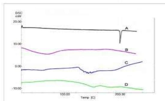
**Fig 8: Overlaying of DSC thermograms of (A) FBX, (B) Soluplus, (C) Physical mixture, (D) solid dispersion**
