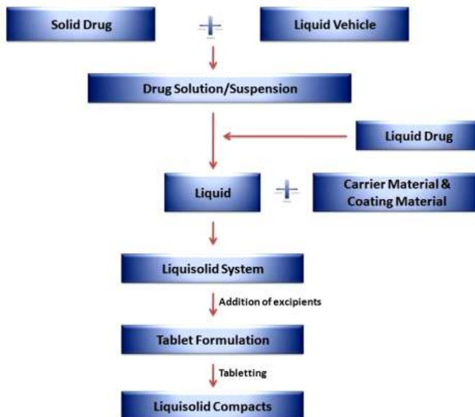
**Fig: Flow chart of the steps involved in the preparation of liquisolid compacts.**
