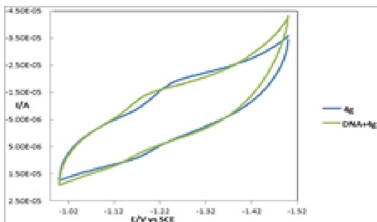
**Figure 9: Cyclic Voltammogram for (0.1M) D at Scan Rate of 0.2V/s in Ethanol Water Mixture (8:2) at pH 7.4.**
