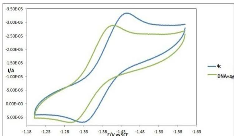
**Figure 7: Cyclic Voltammogram for (0.1M) B at Scan Rate of 0.2V/s in Ethanol Water Mixture (8:2) at pH 7.4.**
