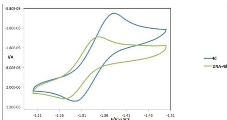
**Figure 8: Cyclic Voltammogram for (0.1M) C at Scan Rate of 0.2V/s in Ethanol Water Mixture (8:2) at pH 7.4.**
