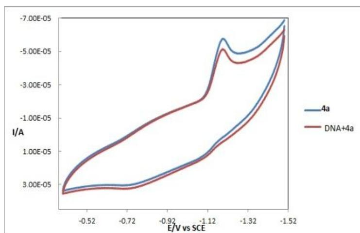
**Figure 6: Cyclic Voltammogram for (0.1M) A at Scan Rate of 0.2V/s in Ethanol Water Mixture (8:2) at pH 7.4.**
