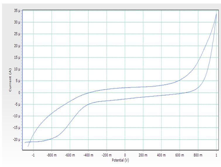
Fig. 9 Cyclic voltammogram of [Co(HEDTA)N<sub>3</sub>]<sup>-</sup> complex
