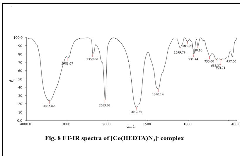
Fig. 8 FT-IR spectra of [Co(HEDTA)N<sub>3</sub>]<sup>-</sup> complex
