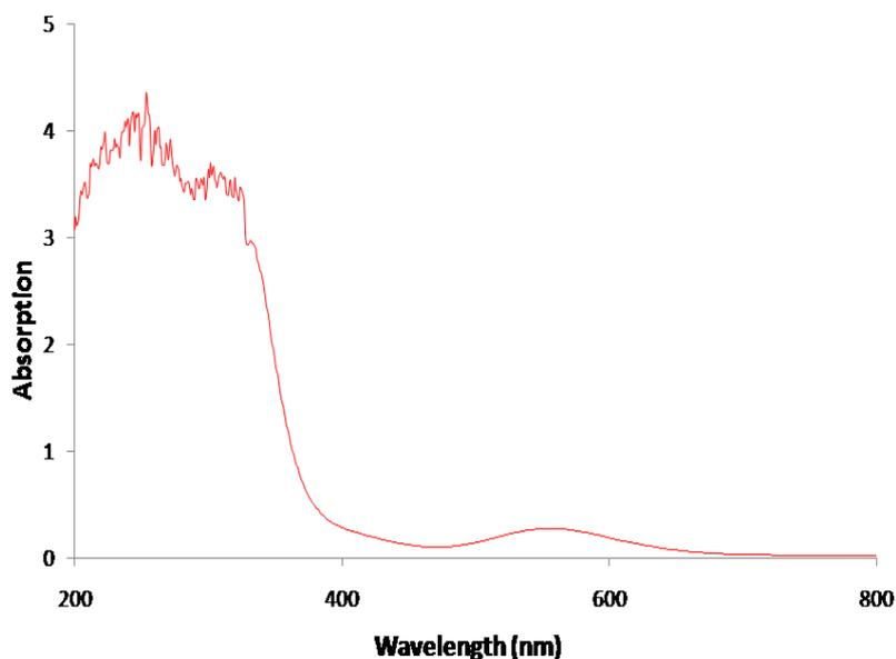
**Fig. 7 UV-Visible spectra of  $[\text{Co}(\text{HEDTA})\text{N}_3]^-$  complex**
