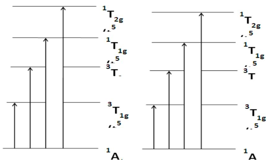
**Fig. 6 Energy Level Diagram for the Ligand-field States of Octahedral Cobalt (III) Complexes**
